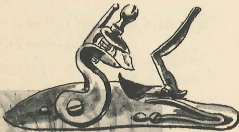
The snaphaunce lock (left) like the wheel lock before, led to the development of better hand guns.
